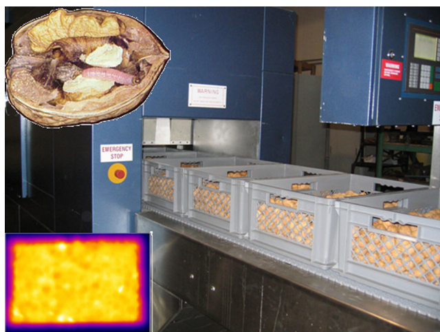
Fig. 1 Photo of infested walnut (inset, top left) of an industrial-scale radio frequency system (Wang et al. 2007) and an infrared thermal (IR) image of walnut surface temperatures in a plastic container after radio frequency treatment (inset, bottom left)
