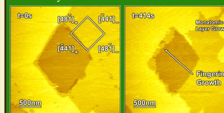
Fingered growth (as indicated by the white arrow) appears to be growing normal to the edge of the fast steps in the etch pit. The images were obtained at a normal force of 17 nN and a scan speed of 2.2  $\mu$ m/s. The scan on the left was taken in a solution concentration of  $\sigma = 0.7$  and the image on the right was placed in a more saturated solution of  $\sigma = 1.42$ , the new growth is shown by the arrow.
