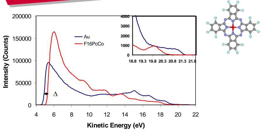
A vacuum shift  $\Delta = 0.5$  eV was measured at the lower KE side of the UPS spectrum obtained for the compound.
