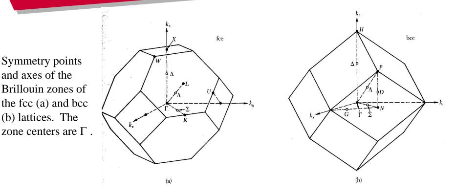
In (a) the boundary point at  $2\pi/a$  (001) is X; the boundary point at  $2\pi/a$  (1/2,1/2,1/2) is L, the line  $\Delta$  runs between  $\Gamma$  and X.
