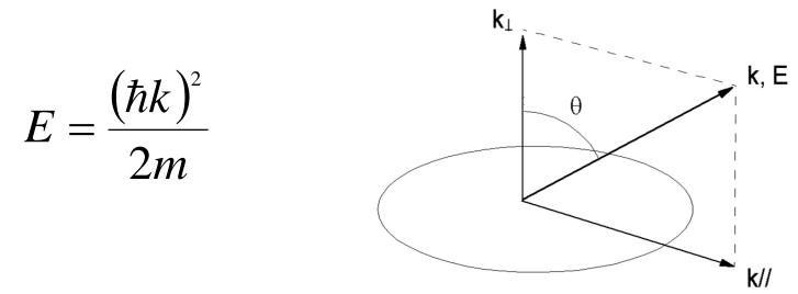
The knowledge of E and then  $|k_i\rangle$  allows one to get the band structure diagram  $E \rightarrow k$  (wavevector).
