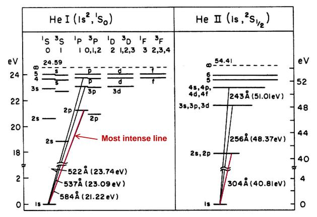
Grotian diagram for He I and He II showing the strongest resonance lines (584 Å, 98% of the emission intensity, the other lines present in a He discharge are 537 Å, 522 Å and 304 Å which can have intensity of the order of 2 % of the 584 Å line. *Rabalais J. Wayne "Principle of Ultraviolet Photoelectron Spectroscopy", John Wiley&Sons Inc.* 1977.
