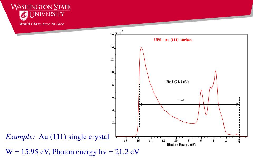
$\phi_m = 21.2 - 15.95 = 5.25 \text{ eV} \pm 0.15 \text{eV}$  (resolution of the instrument) Literature value 5.3 eV (CRC)
