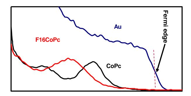
UPS data shows the first ionization energies for CoPc and  $F_{16}$ CoPc (HOMO) adsorbed on Au surface. A difference of 0.5 eV was measured between CoPc and F16CoPc compounds. This is due to the high electro-negativity of fluorine (highest withdrawing electron power than of H) therefore the electrons are tightly bound  $\rightarrow$  need more energy (higher KE).
