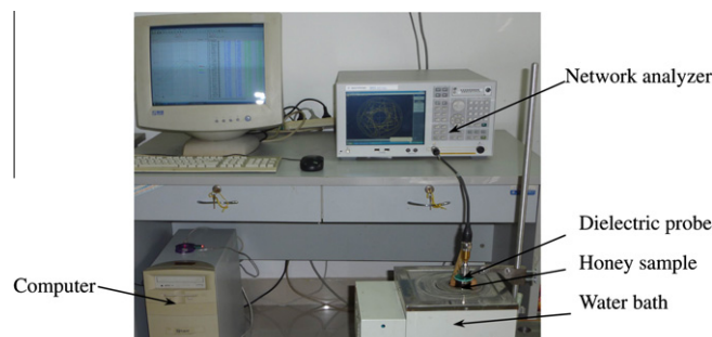
Fig. 1. Dielectric properties measurement system.
