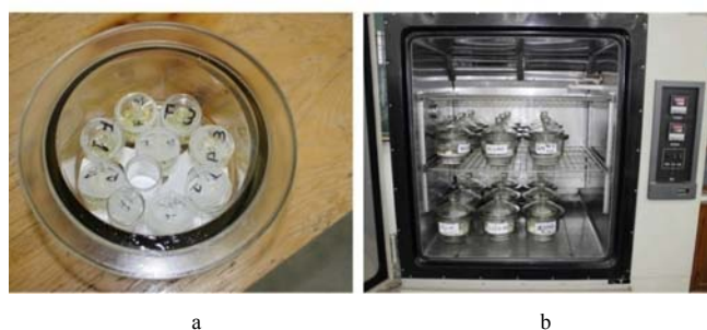
Figure 2 Sealed desiccators (a) and temperature controlled incubator (b) used in the experiments
